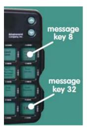
Function mode allows you to change the settings on the device. The settings on the device that can be changed are printed on the green membrane that shows under the keyguard grid. The top row lists the settings that effect the overall operation of the device. The bottom three rows change the scanning settings (see Scanning Access below). The available operational settings on the top row include:
